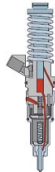
A new generation of electronically controlled high pressure unit injectors for precise fuel injection timing and fuel quantity delivery for each combustion sequence.
